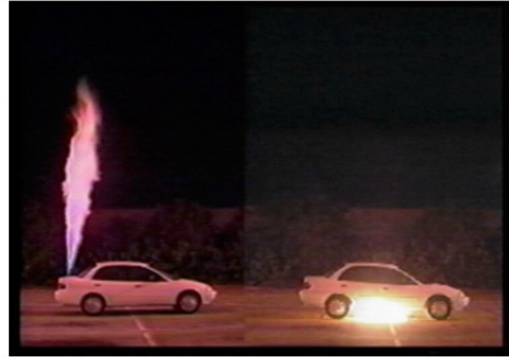
Photo 2 - Time 0 min, 3 seconds - Ignition of both fuels occur. Hydrogen flow rate 2100 SCFM. Gasoline flow rate 680 cc/min.
